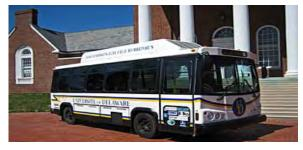
The University of Delaware's Department of Mechanical Engineering conducts research on two fuel cell buses that operate along normal campus routes. The 20 kW fuel cells are from Ballard Power Systems.
