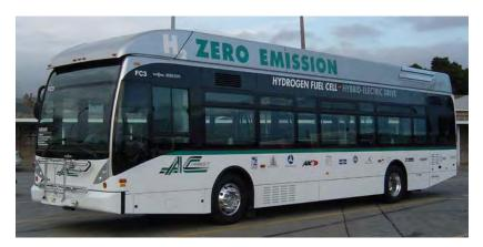
AC Transit has partnered with UTC Power to place three fuel cell buses on the road in California, with 12 more buses planned.
